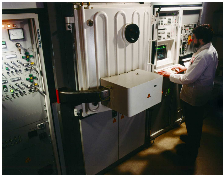
Newport's Stabilife Reactive Ion Plating Deposition System
